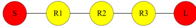
Fig. 6. Coupling topology of the third-order filter. (R1, R2, R3, S, and L denote the feeding network, the coupling slot, the antenna unit, the source, and the load, respectively.)
